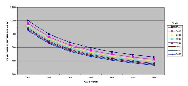
It is unlikely that "worst in class" later generation mines achieving say ≥100m per week per continuous miner, or in the case of super unit mines ≥130m per week per super unit, could reasonably sustain 15Mtpa longwall mines (mining heights 3.0 to 4.0m), unless longwall block lengths and face widths were extended to or beyond current technological limits.
