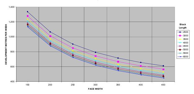
EFFECT OF FACE WIDTH AND BLOCK LENGTH ON WEEKLY DEVELOPMENT RATES - 4.0m MINING HEIGHT 15Mtpa
