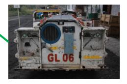
EPOD/RPOD's installed on rear of vehicle in a protected position.
